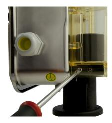
**E** Remove the screw blocking the Reed contact.
