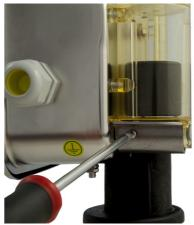
Ž Insert the screw supplied with the antimagnetic shield in the hole and screw it with a Philips screwdriver.
