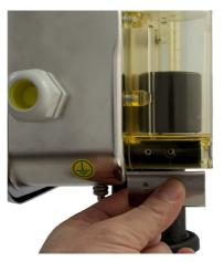
• Position the antimagnetic shield making sure that both the antimagnetic shield and the Reed housing's holes are aligned.
