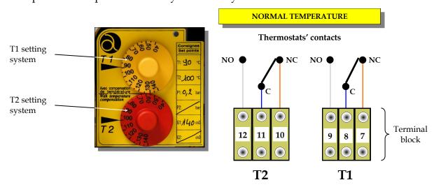
When the dielectric temperature reaches the set-point value (±2.5°C), the thermostat's contact changes position.
