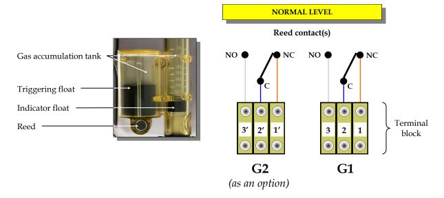
When the gas volume inside the gas accumulation tank reaches a certain value (depending on the dielectric density), the Reed contact changes position.
