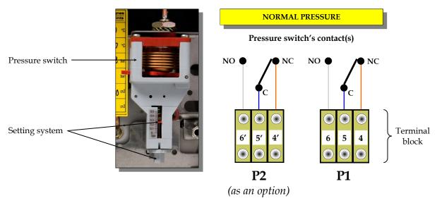
When the tank pressure reaches the set-point value (±0.01 bar), the pressure switch's contact changes position.
