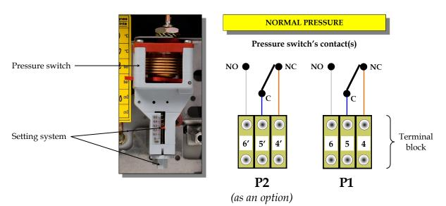
When the tank pressure reaches the set-point value, the pressure switch's contact changes position.
